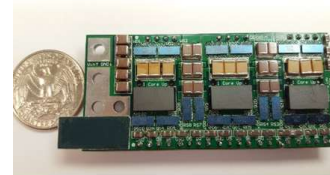
600W GaN DC-DC Converter 99% efficiency
