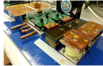
100 kW SiC Power Converter 42 kW/L 99% efficiency
