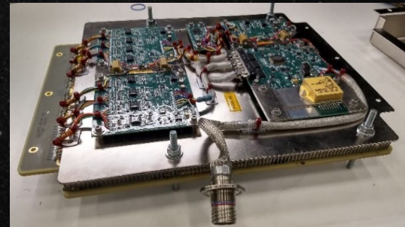
Power Management Electronics for a Lunar Surface Testbed
