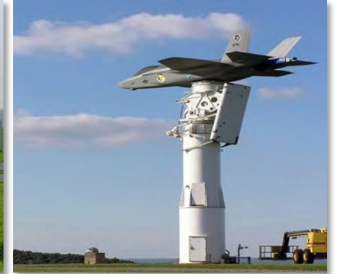
Outdoor Antenna Test Ranges
